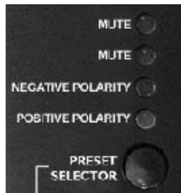
Figure 8: SB15P preset selector switch closeup
