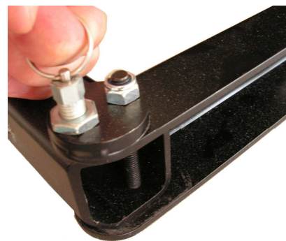
(4) Release pivoting arm locking pin
